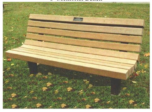
The contoured supports are 3/8" x 4" rolled steel, shaped to provide a smooth, comfortable seat and backrest. The legs are 2- ½" square steel support tubing, welded to an arched 3/8" x 4" formed steel base. The frame is coated black for durability and an attractive appearance. The slats are 4" x 4" cedar-color recycled plastic. The bench is mounted directly into the ground, and each leg is anchored with concrete.
