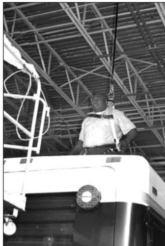
Palm Tran Mechanic Babatunde Atoki wears the new harness while working on top of a bus.
