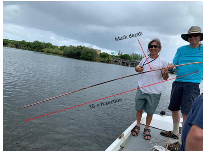
Figure 3 Sediment bottom gauge (Site 125).
