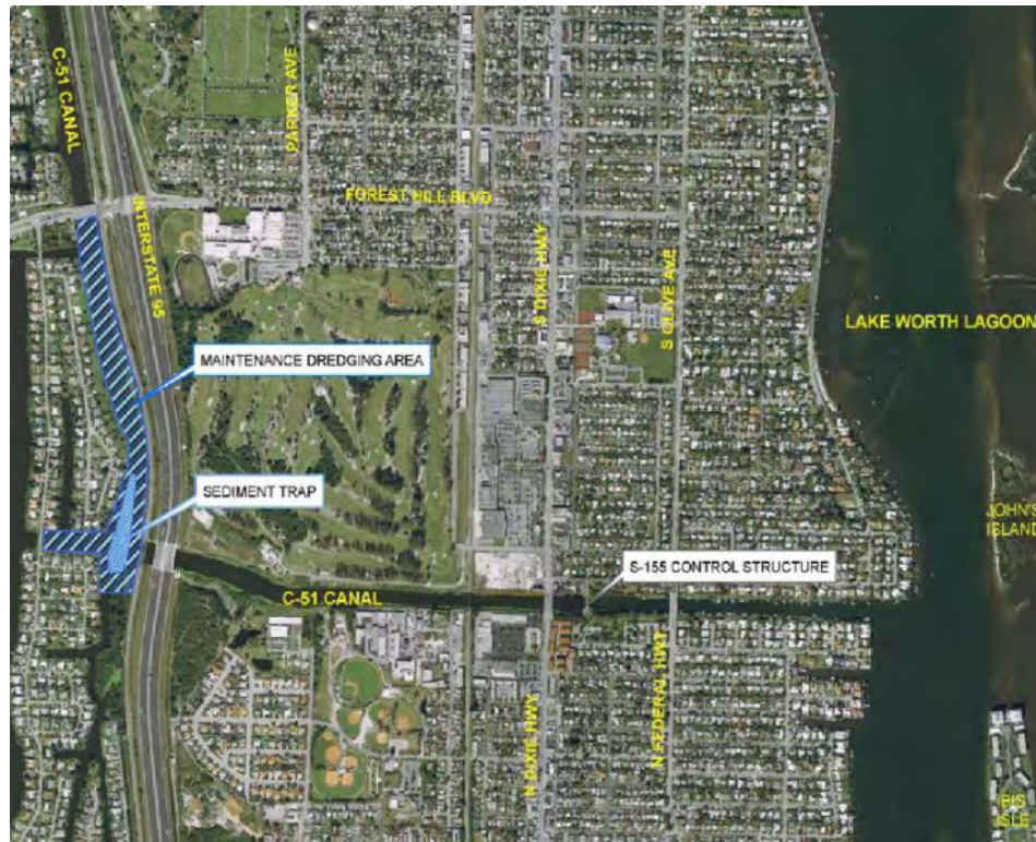
Figure 1 Location of C-51 Canal Sediment Trap
