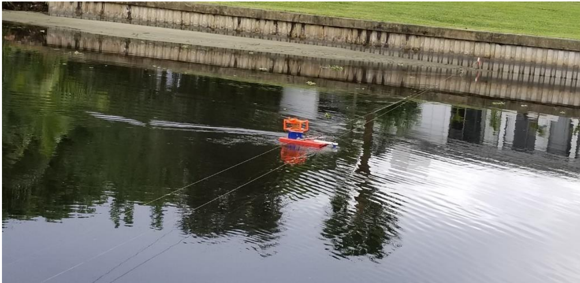
Figure 6 Stream gauging using a tag line at a Transect.
